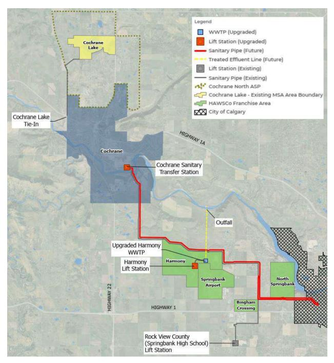
Figure 7: Option 2A - Status Quo with Harmony WWTP Outfall Upstream of Bearspaw WTP Intake
