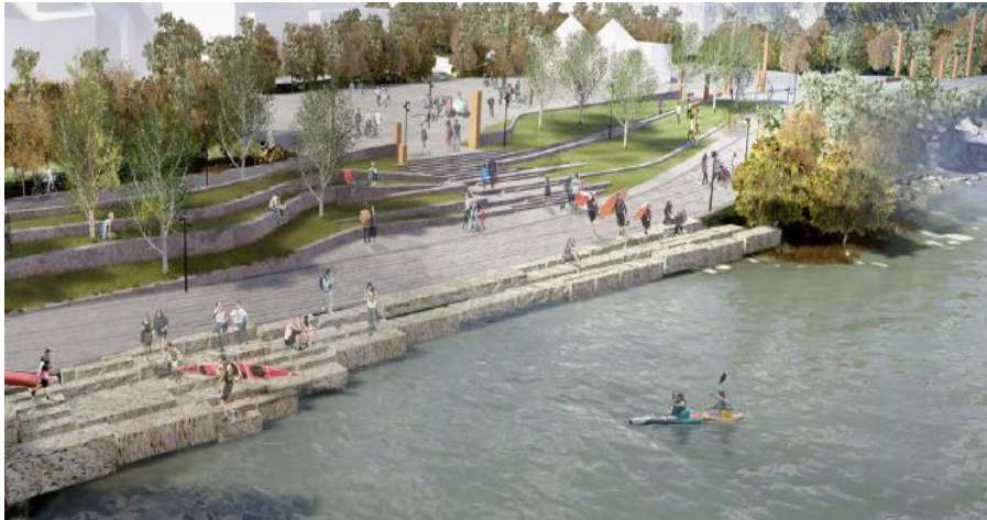
CONCEPTUAL DESIGN OF THE EAU CLAIRE PROMENADE, WHICH INCLUDES THE DOWNTOWN FLOOD BARRIER. FLOOD MITIGATION WILL CONNECT WITH THE FLOOD BARRIER IN WEST EAU CLAIRE PARK TO GREATLY REDUCE FLOOD DAMAGE RISK IN CALGARY'S DOWNTOWN. THIS PROJECT IS BEING COMPLETED WITH SUPPORT FROM THE PROVINCE THROUGH ITS ACRP PROGRAM.
