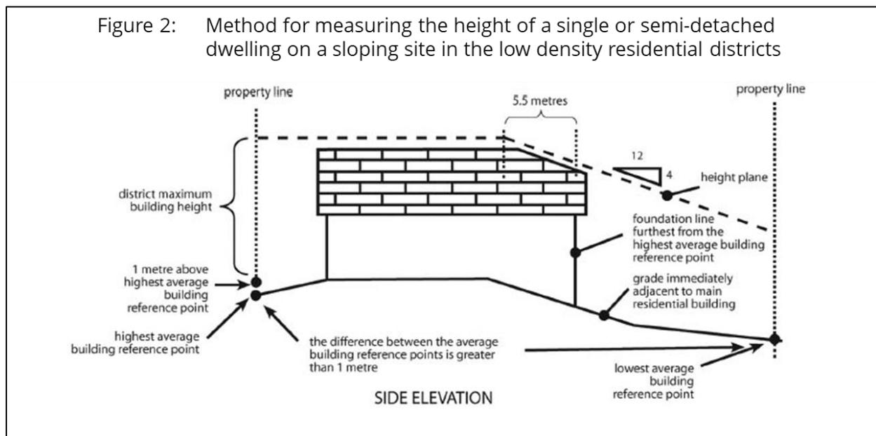
Figure 3: Method for measuring height of a single detached dwelling on a sloped parcel
