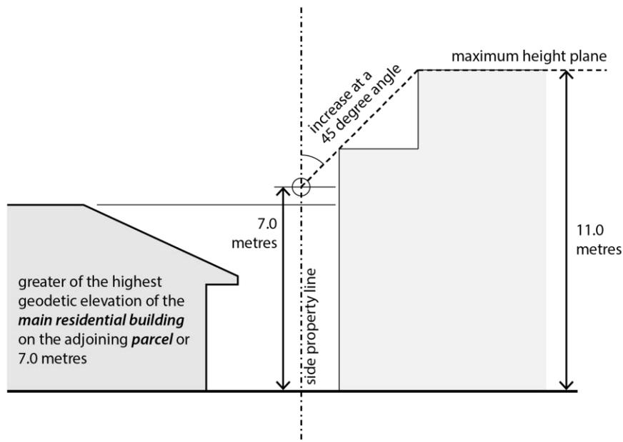
Figure 7: Proposed height chamfer on a corner parcel
