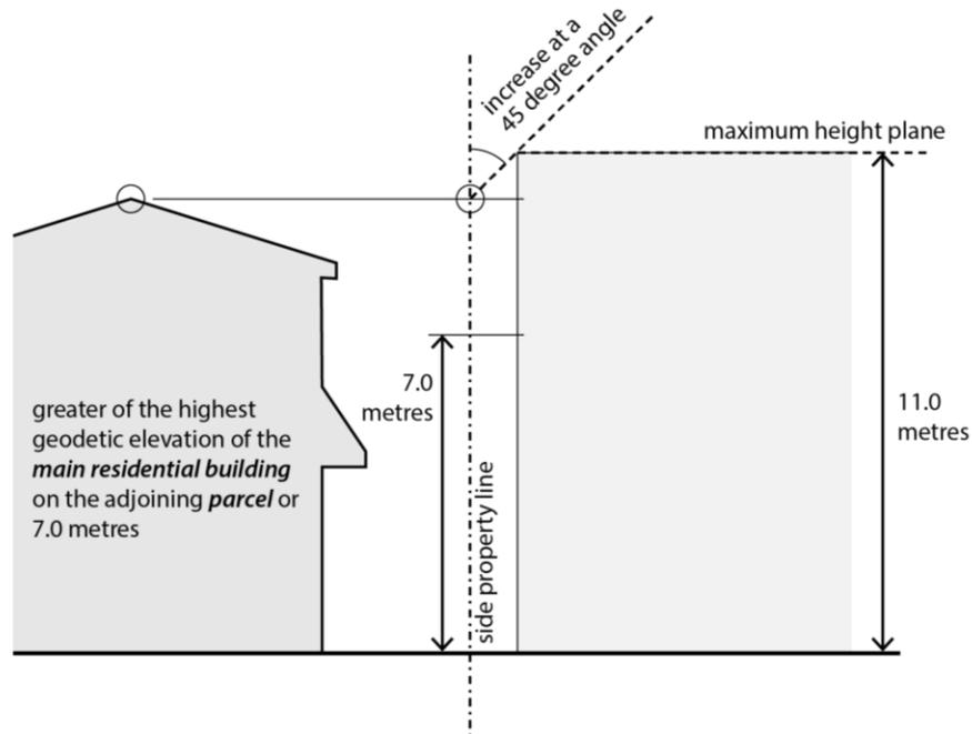
Figure 6: Proposed height chamfer next to a building under 7 metres
