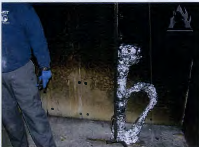
Figure A-4: Heat Flux Gauge with Radiation Shielding
