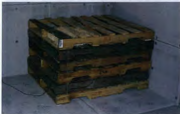
Figure A-2. Pallets and Excelsior Ignition Source Used as a Fuel Source
