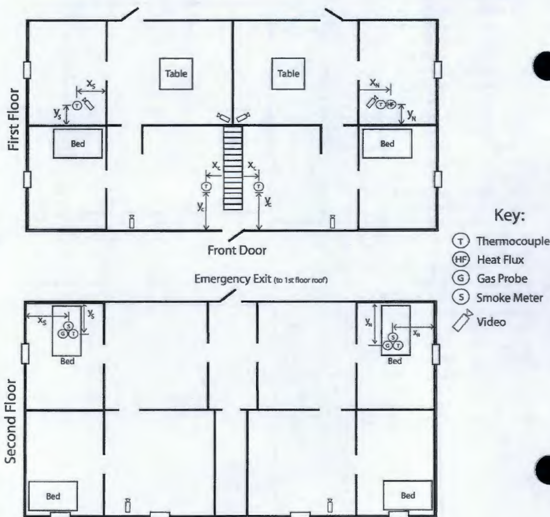
Figure 6: Instrumentation and Furniture Prop Layout
