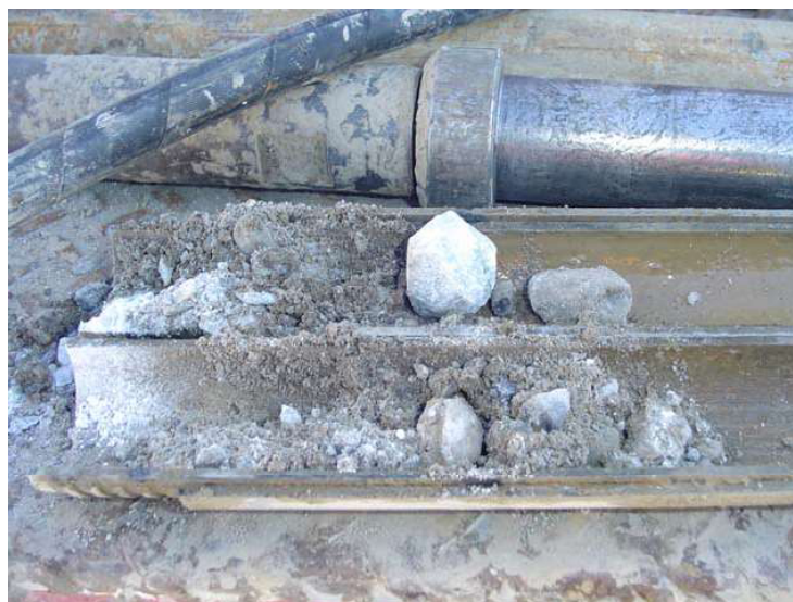
Photo 3: Sand and gravel fill from 600 to 760 mm depth in BH02
