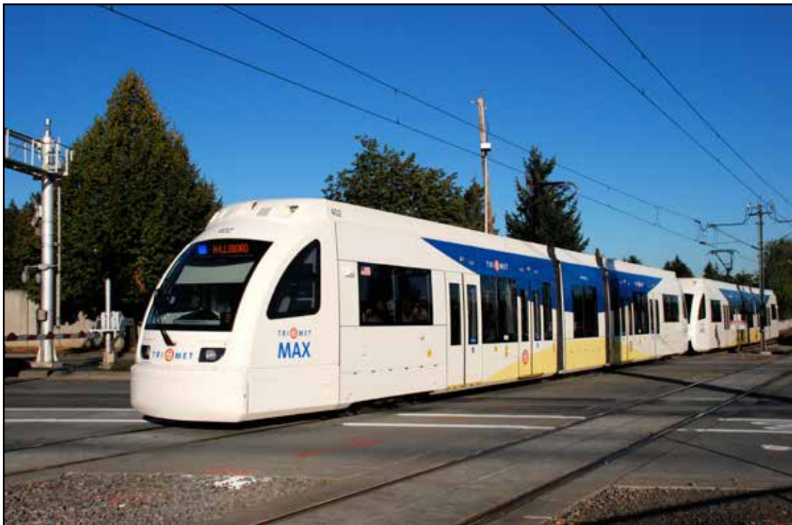
Siemens S70 low-floor cars, Portland MAX system
