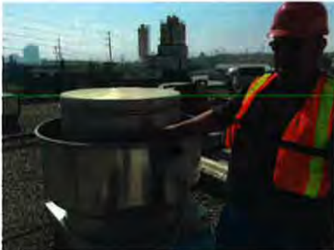
Photo 1 – Live Shed: Odour sample collected at approximately chest height at an exhaust ventilation louvre immediately prior to air exiting the louvre to the outside of the building along the northeast wall at the approximate mid-point of the building's southwest face.
