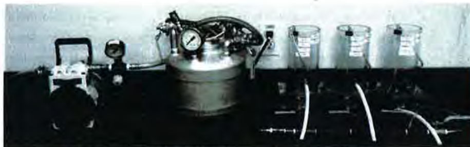
Figure 2: Dissolved air flotation (DAF) laboratory bench testing apparatus
