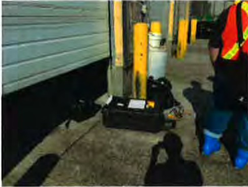
Photo 1 – Live Shed: Odour sample collected at approximately chest height at an exhaust ventilation louvre immediately prior to air exiting the louvre to the outside of the building along the northeast wall at the approximate mid-point of the building's southwest face.
