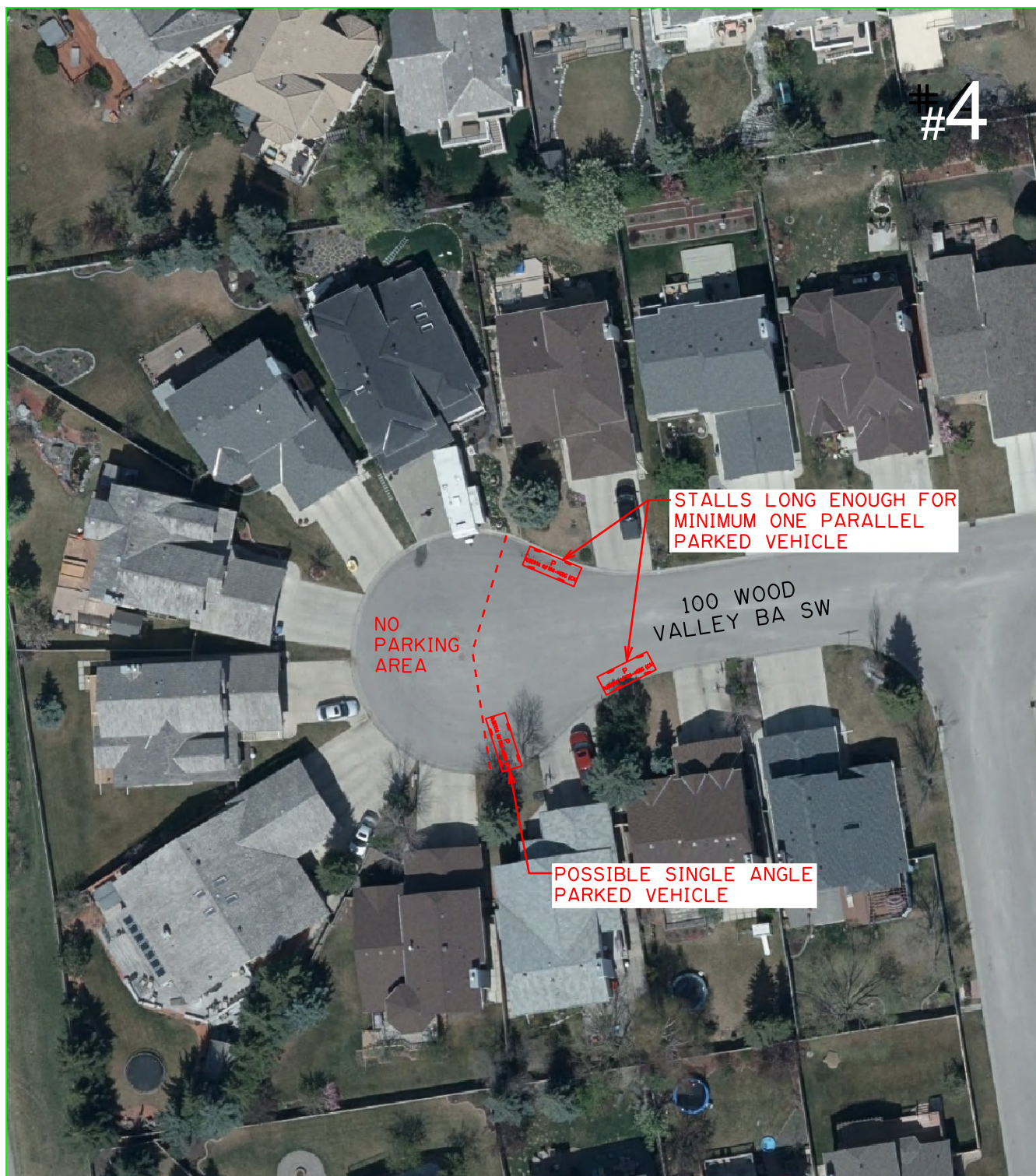
TYPICAL CITY OF CALGARY RESIDENTIAL STREET CUL-DE-SAC DESIGN (BULB RADII VARY)
