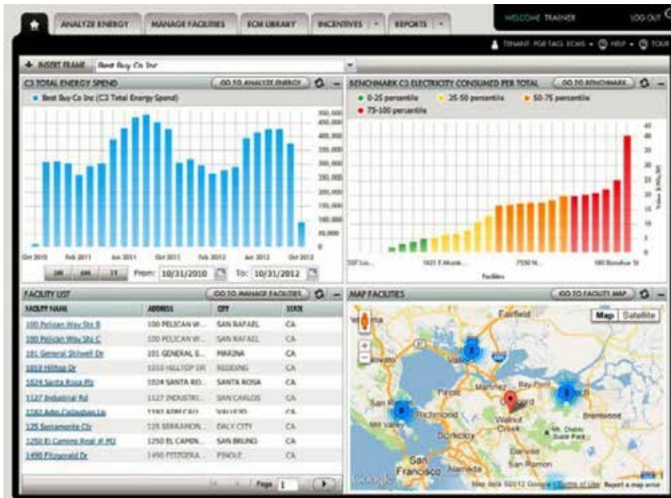
Figure 4 – Web-based Energy Portal from C3 Energy displaying the energy use of multiple facilities from one organization in a certain geographical area
