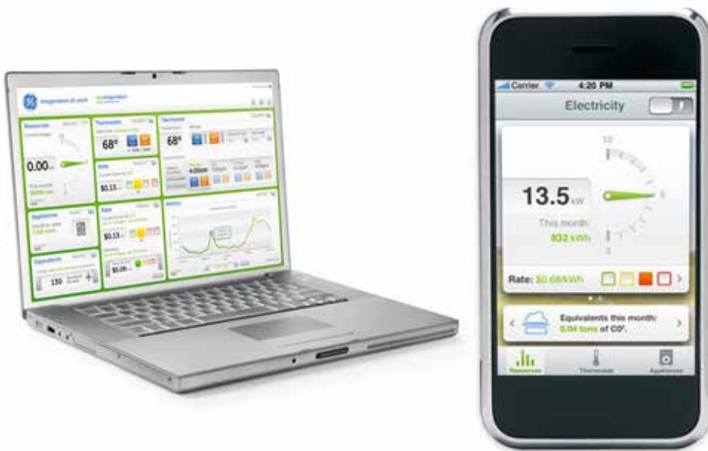
Figure 3 – GE offers an energy display that communicates with the utility smart meter to provide consumers with near real-time energy data.
