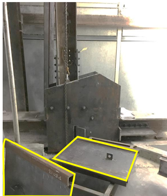
Example of Steel plates prior to installation; “Stiffeners”
