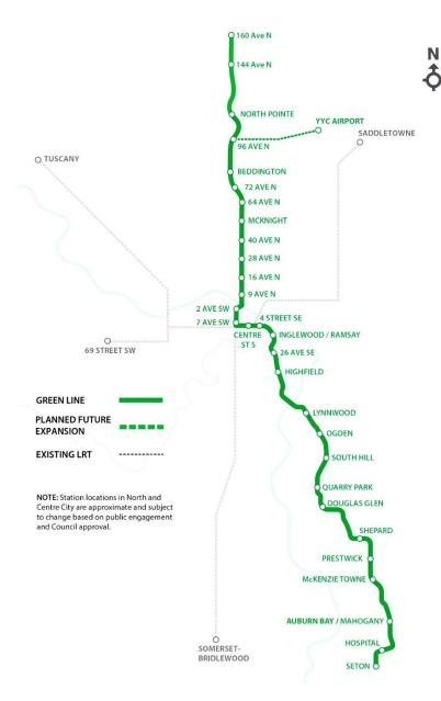
At full community build-out, the Green Line is expected to carry an estimated 240,000 trips per day. The final route will stretch 46 km from 160 Avenue North to Seton in the Southeast and connect 28 stations. The Green Line was designed to be delivered in stages with completion of stage I (16 Avenue North to 126 Ave Southeast) scheduled for 2026 at an estimated construction cost of \$4.65B, based on a Class 3 capital estimate <sup>2</sup>.
