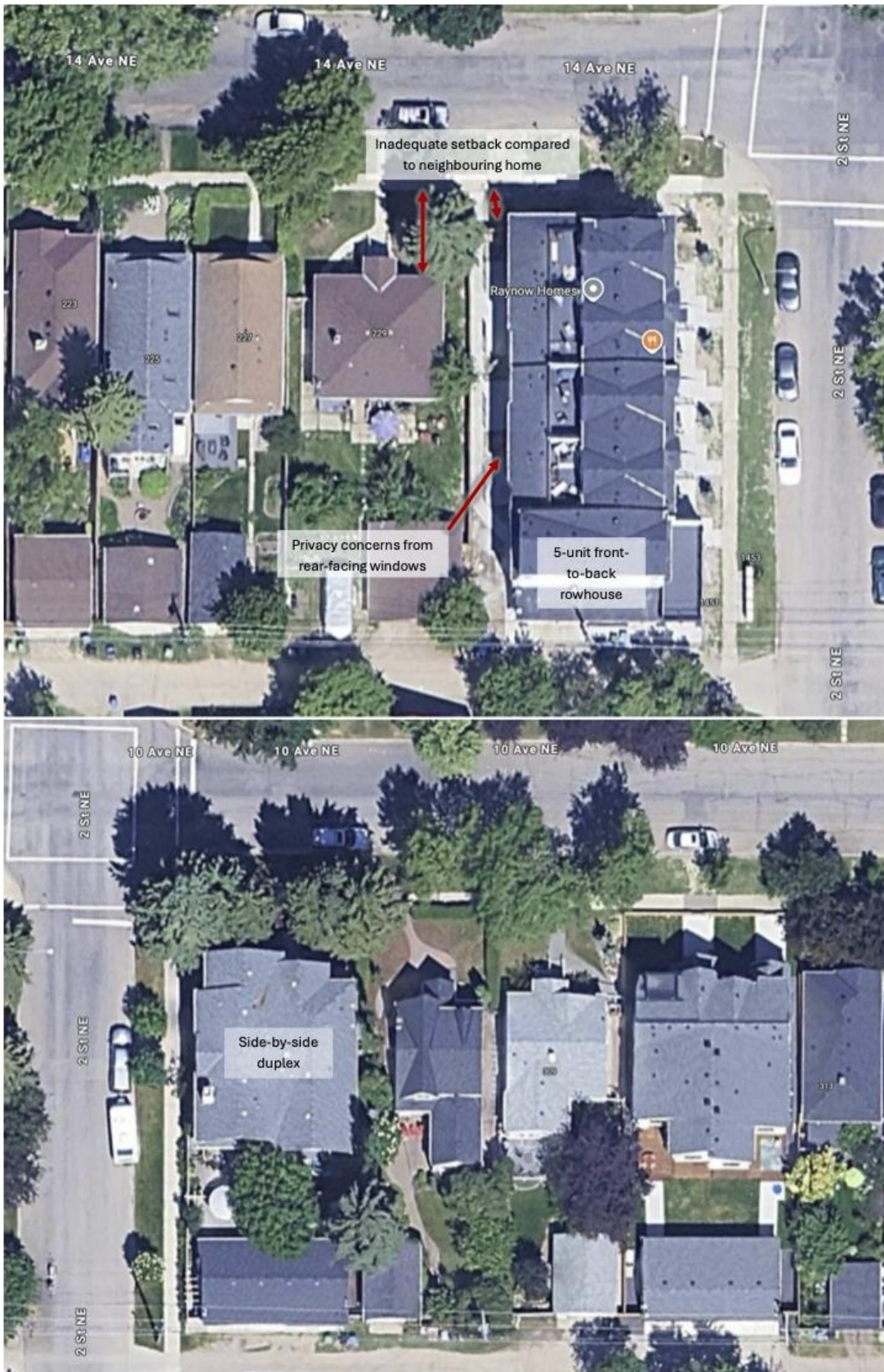
Figure 3 Front-to-back development (top) compared to side-by-side development (bottom). Privacy and setback concerns highlighted in front-to-back development
