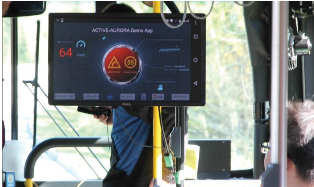
Figure 2: As part of the ACTIVE AURORA project, The City of Edmonton outfitted one of its buses with connected vehicle technology. The bus can receive audible message warnings that it is speeding, approaching a high collision intersection and if it is following too close (if the vehicle ahead is equipped with connected vehicle technology).
