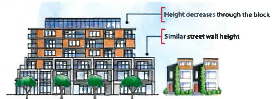
(above) Illustrative guidance from the Riley LAP showing meaningful step-backs above the 3 rd storey
