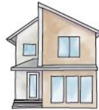
Contemporary asymmetrical roof
