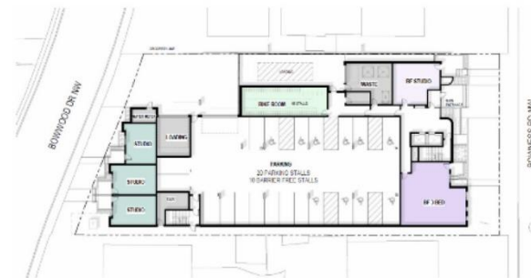
Figure 7: Preliminary ground floor schematic showing parking
