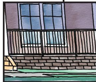
Heavier materials at base of building
