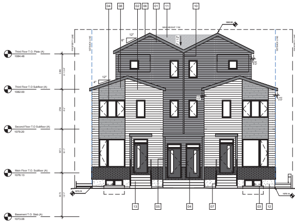
1 BUILDING @ FRONT (SOUTH ELEVATION) 3/16" = 1'-0"
