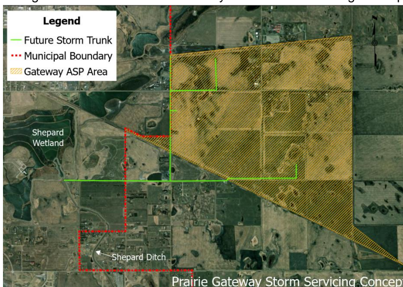
Figure 1: Potential Prairie Gateway Stormwater Servicing Concept
