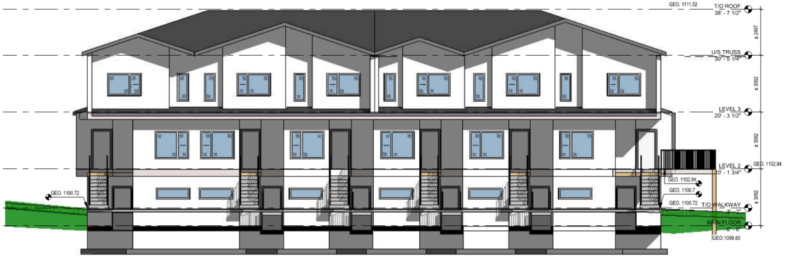
1 BUILDING#1 FRONT ELEVATION DP-101 | 1:100
