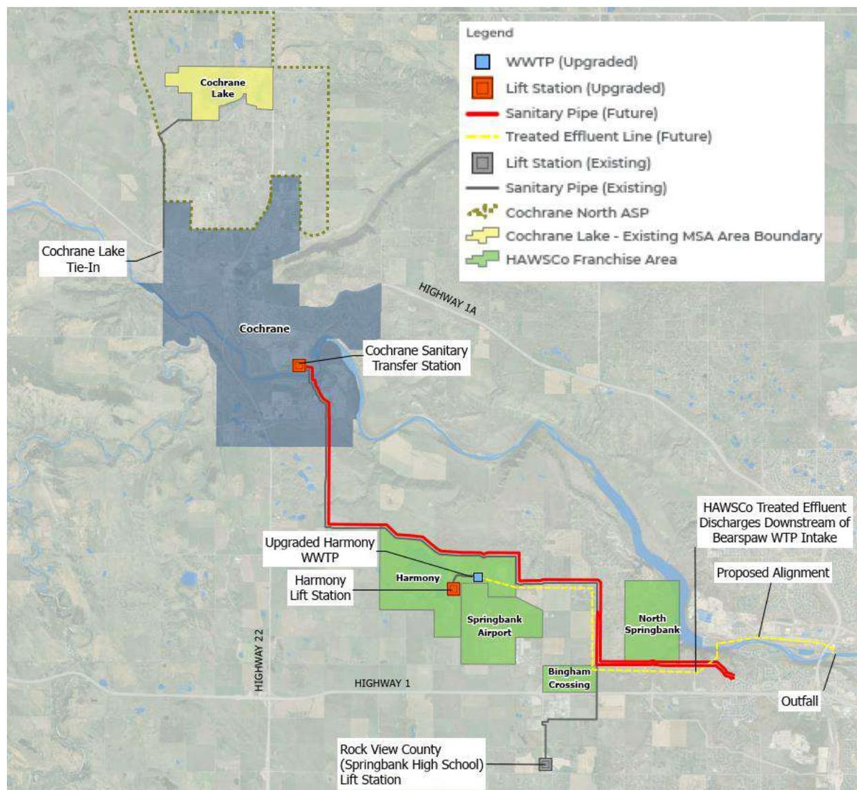
Figure 8: Option 2B - Status Quo with Harmony WWTP Outfall Downstream of Bearspaw WTP Intake
