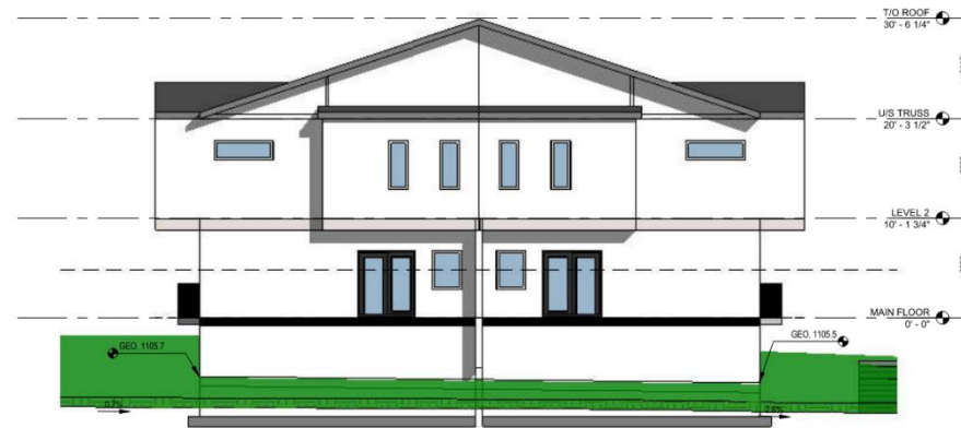
4 BUILDING#17 SIDE ELEVATION DP.117 1:100
