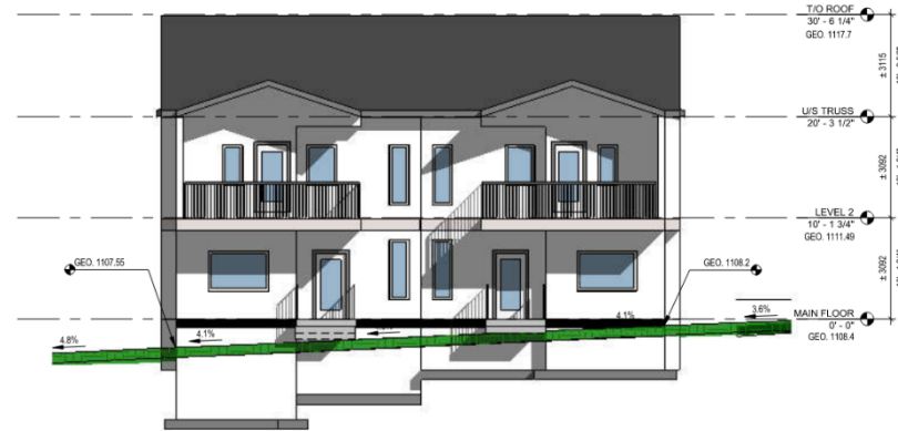
1 BUILDING#15 SIDE ELEVATION DP.115 1:100
