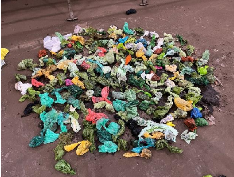
Image 10: Pet waste from diversion pilot at Calgary Composting Facility – highly contaminated with plastic pet waste bags.
