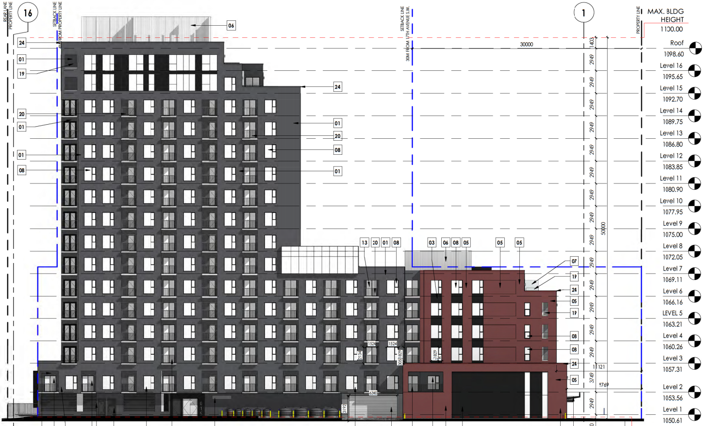
2 EAST COLOUR ELEVATION DP3.05 1 : 200
