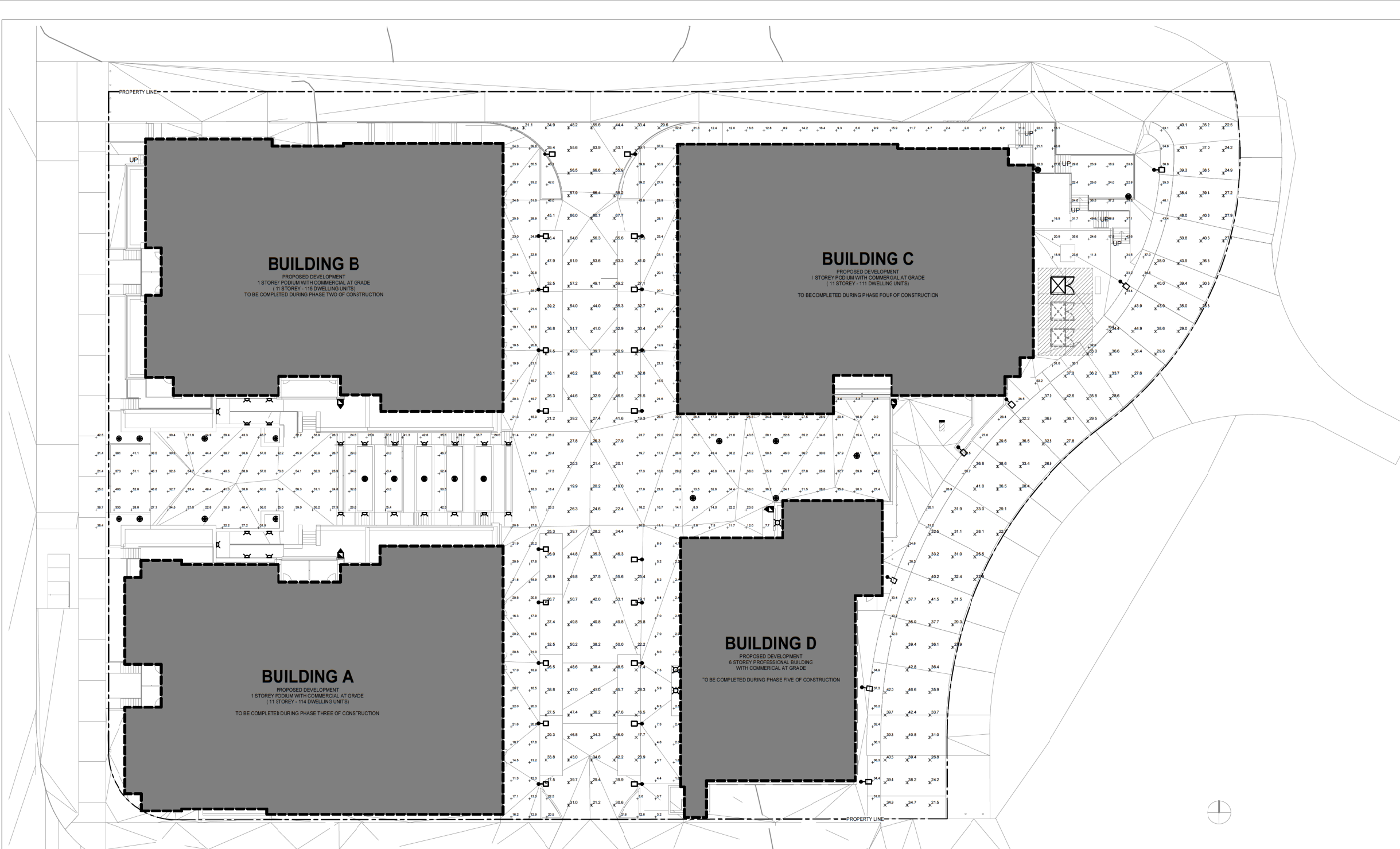
1 DP LIGHTING POINT-BY-POINT DPE1.2 Scale: 1:200
