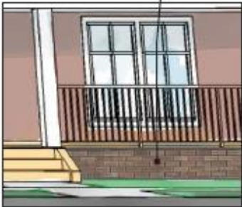
Heavier materials at base of building
