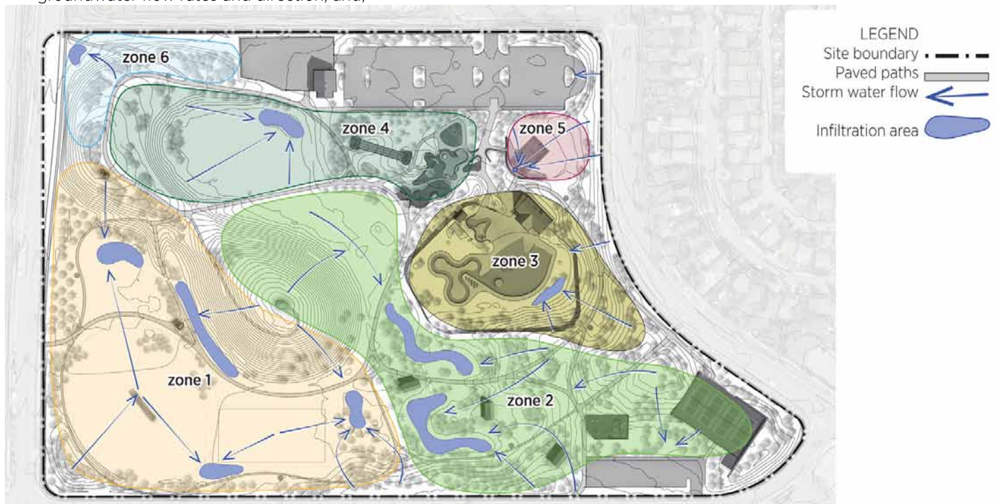
FIGURE 7.27: CONCEPTUAL STORMWATER MANAGEMENT SCHEMATIC
