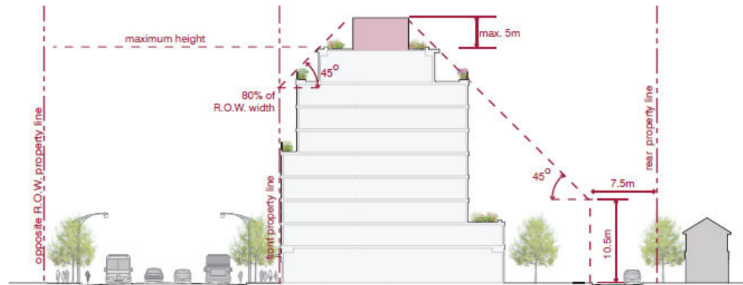
Example of mechanical penthouse placement within all angular planes.
