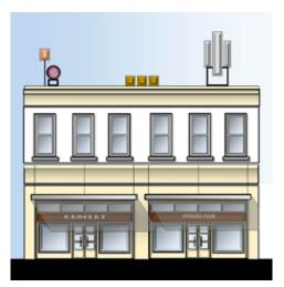
Conspicuous installations above the parapet are discouraged.
