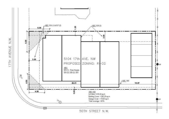
Next, on the following diagram we demonstrate a typical R-CG layout on a corner lot showing where the above bylaws are applicable and noted on the drawings.
