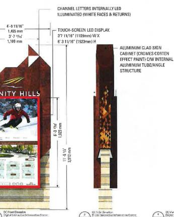
ALLANSON STORMTIGHT WHITE LEDS ON 4" CENTRES, CV125-120 POWER SUPPLIES, ALLANSON TRANSFORMERS AND BX CABLE TO BE FULLY CONCEALED
