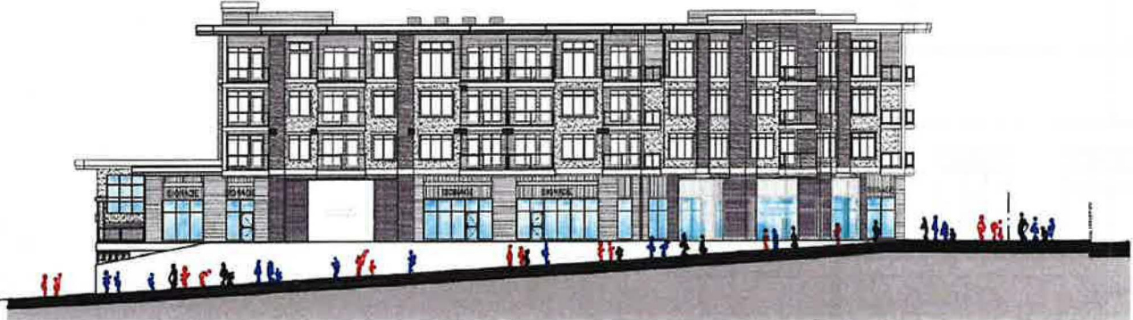
C 19TH AVENUE SW - GRADES ALONG WALKWAY WITH MAIN FLOOR LEVEL WITH 85TH STREET SW LESS THAN HALF OF THE STOREFRONTS ARE VISIBLE TO PEDESTRIANS
