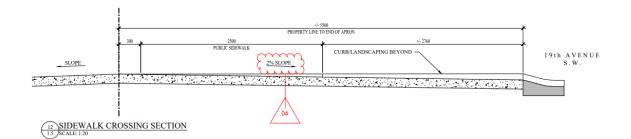
**NOTE:** Although the boulevard grade has been provided, <u>applicant is to also include the slope of the driveway apron</u>, which will be steeper than 2%. Amend plans accordingly.
