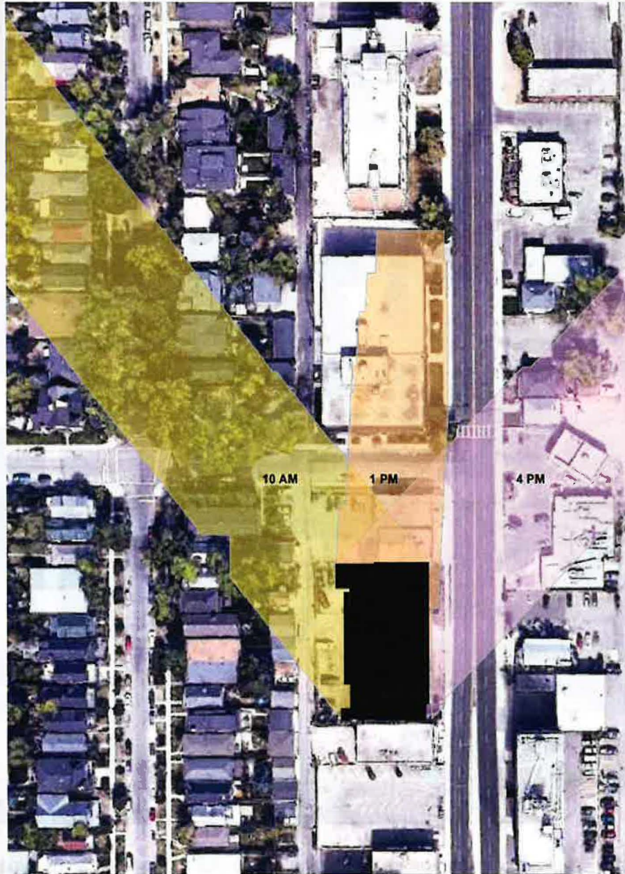
The December 21 shadow created by the proposed building on neighbouring residential to the west is more than the shadow the ARP envelope would create. However for those residences immediately across the lane the impact is still marginally less than the ARP shadow due to the building steps. The shadow impact is greater on lots further away than immediate neighbours. It is meaningful to keep in perspective that the winter sun is predominantly in the south, as such the real impact of shadow created by this building is to the north of the site on 14th street and on other taller buildings where the impact is less of a concern.
