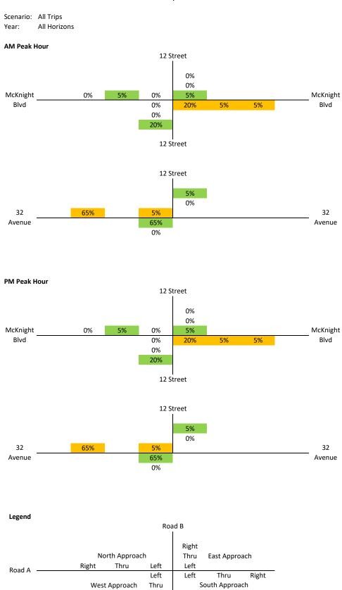
100% Percent of distribution based on total trips 100% Entering trips 100% Exiting trips
