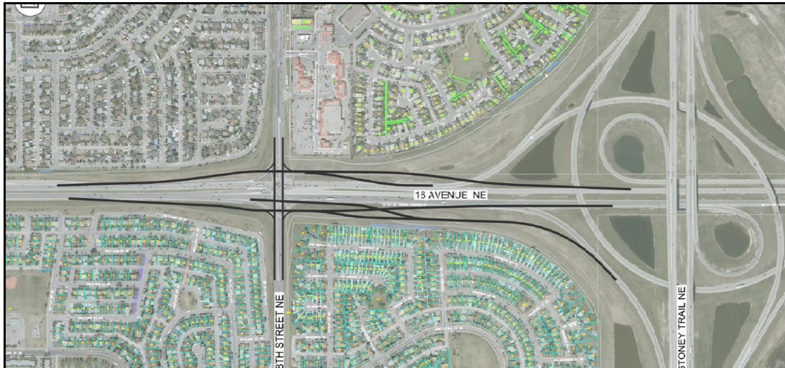
Exhibit 3.1: Diamond Interchange with Basket Weave Structures
