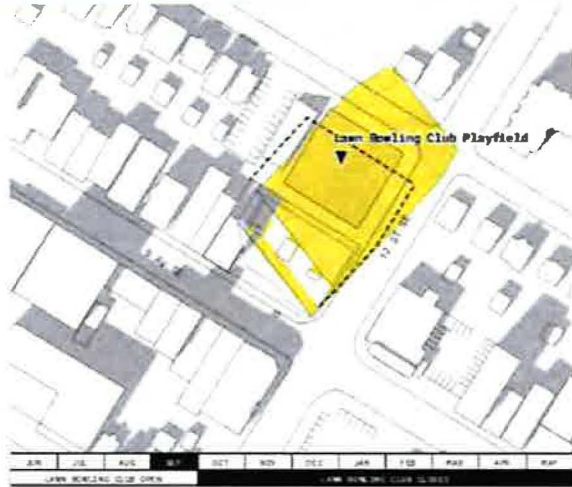
LEGEND [Yellow Box] Proposed Building Shadow [Dashed Line] Existing DC1273 Max Shadow [Grey Box] Existing Built Form Shadow
