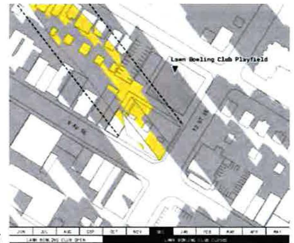
LEGEND [Yellow Box] Proposed Building Shadow [Dashed Line] Existing DC1273 Max Shadow [Grey Box] Existing Built Form Shadow
