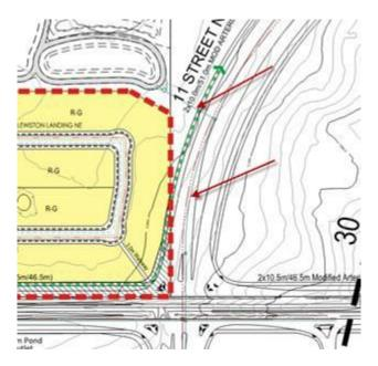
b) The future 144<sup>th</sup> Avenue Storm Trunk will connect to the stormwater facility via a future utility right-of-way through the R-G parcels and/or Lewiston Landing NE located south of the proposed stormwater facility (see figure above).
