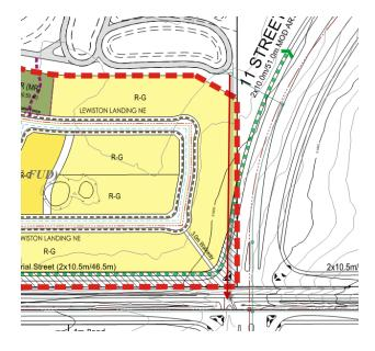
**Prior to endorsement of the tentative plan,** a confirmed alignment of the storm infrastructure required to connect the stormwater facility to the future 144 Avenue Storm Trunk will be required. Note that a utility right-of-way will also be required to be shown on the Lewiston outline plan (currently under review) until such time that an alignment via 11 Street NE has been confirmed.
