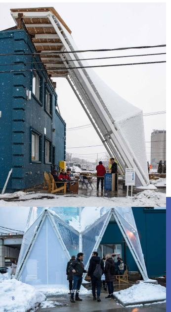
The Raincoat is one of Sidewalk labs many prototypes to provide protection during harsh weather and is one example of the many microclimate innovations in development, working to enhance outdoor comfort year-round in public spaces. The Raincoat consists of an adjustable awning or second skin that could extend outward from a building's edge to protect the sidewalk from rain, wind and sun.
