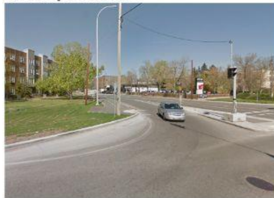
small curve radius, lower speeds, high entry angle
