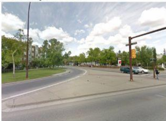
large curve radius, higher speeds, low entry angle
