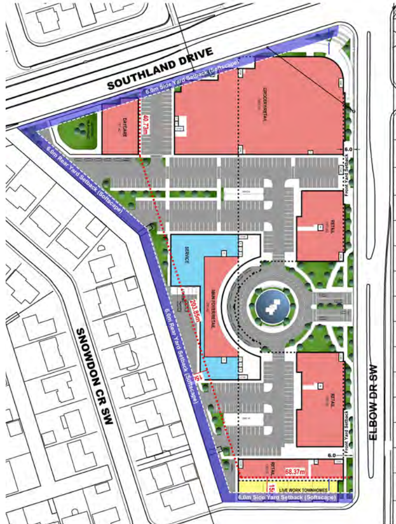
FIGURE 12: ENCROACHMENTS INTO THE REAR AND SIDE YARD SETBACKS SHOWN IN PURPLE ON THE REVISED CONCEPT PLAN. CONCEPT ONLY, SUBJECT TO CHANGE (SABLE DEVELOPMENTS INC.)
