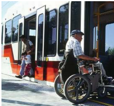
Low floor LRT platform access
