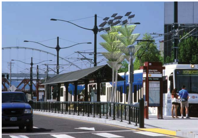
Low floor LRT platform, median transitway
