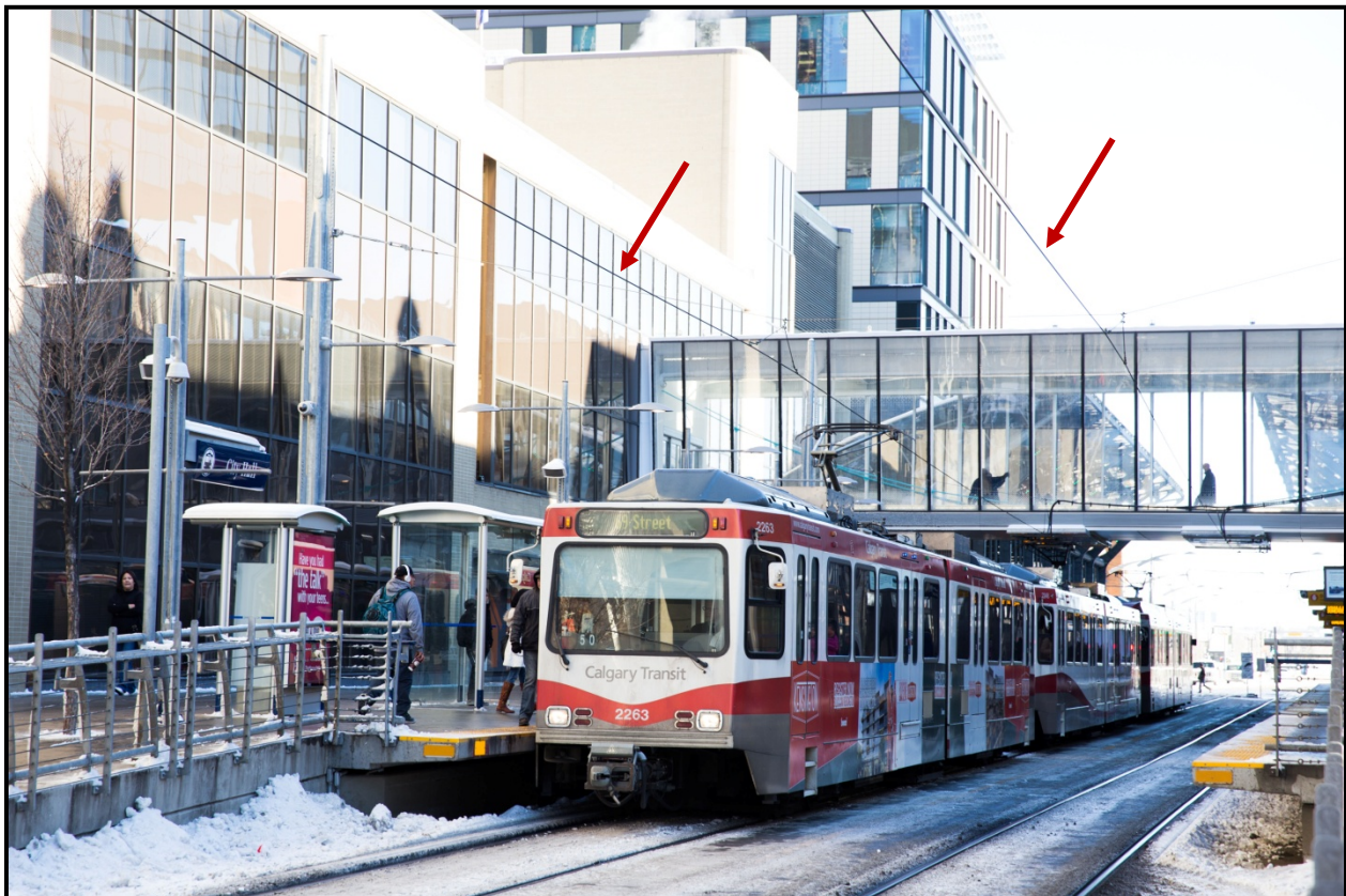
Figure 12: 7 Avenue LRT Catenary Wires (indicated with red arrows)
