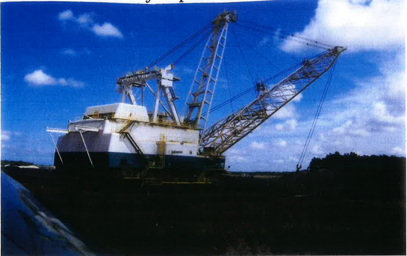
Dragline mining for phosphate at Four Corners Lonesome Mine. Florida's Phosphate Mines
