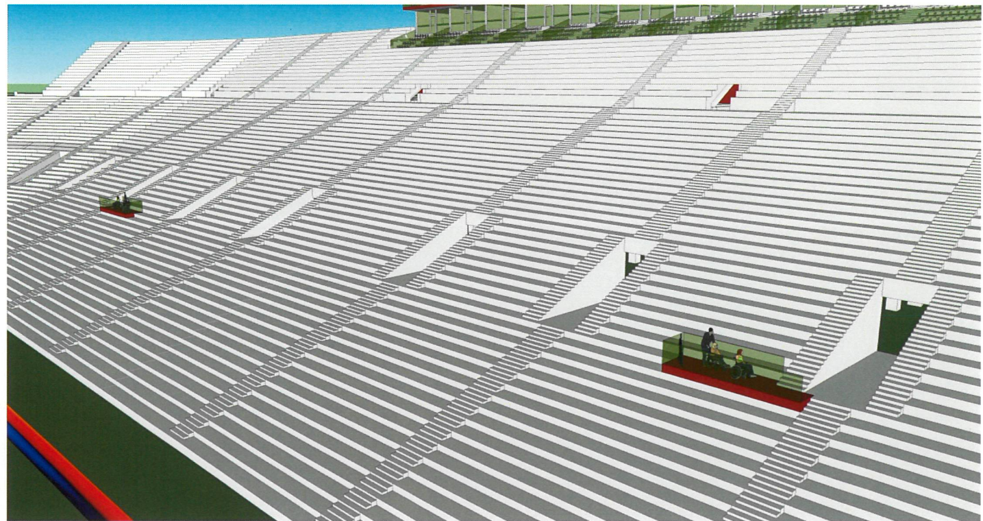
Seating created by absorbing two rows of seats at vomitory level in various locations of the existing grandstands
