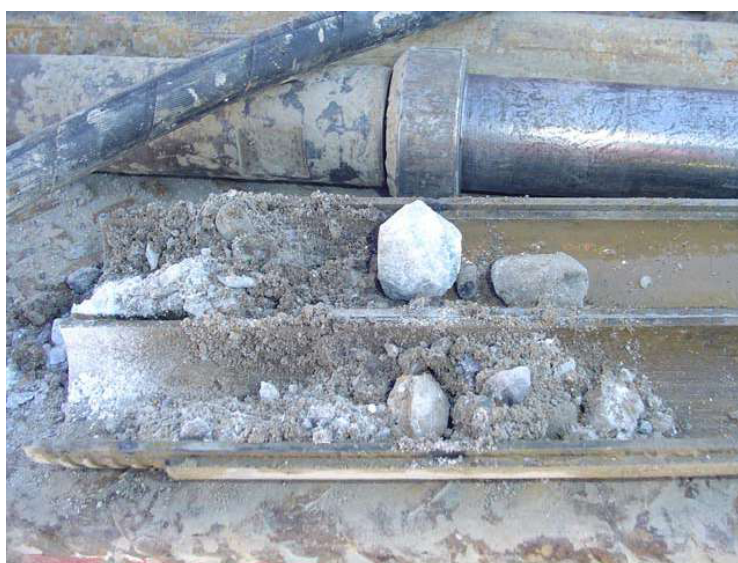
Photo 3: Sand and gravel fill from 600 to 760 mm depth in BH02
