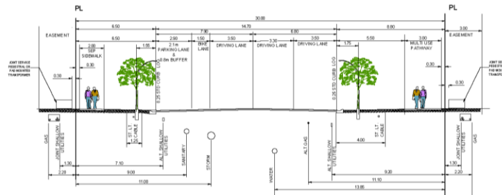
C-C Belmont Boulevard SE (between Belmont View SE and Belmont Avenue SE) Mod. Primary Collector with Multi-Use Pathway 7.90m+6.80m/30.00m
