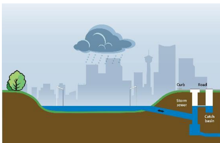
CROSS-SECTION OF A DRY POND. WATER COLLECTED IN A DRY POND DURING A RAINSTORM IS HELD UNDER THE STORMWATER PIPES HAVE THE CAPACITY TO DRAIN THE WATER AWAY. WHEN NOT IN USE, A DRY POND CAN BE USED FOR RECREATION OR LEISURE PURPOSES
