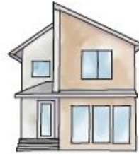
Contemporary asymmetrical roof
