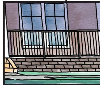
Heavier materials at base of building
