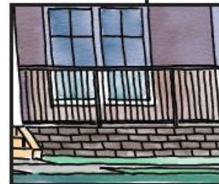
Heavier materials at base of building
