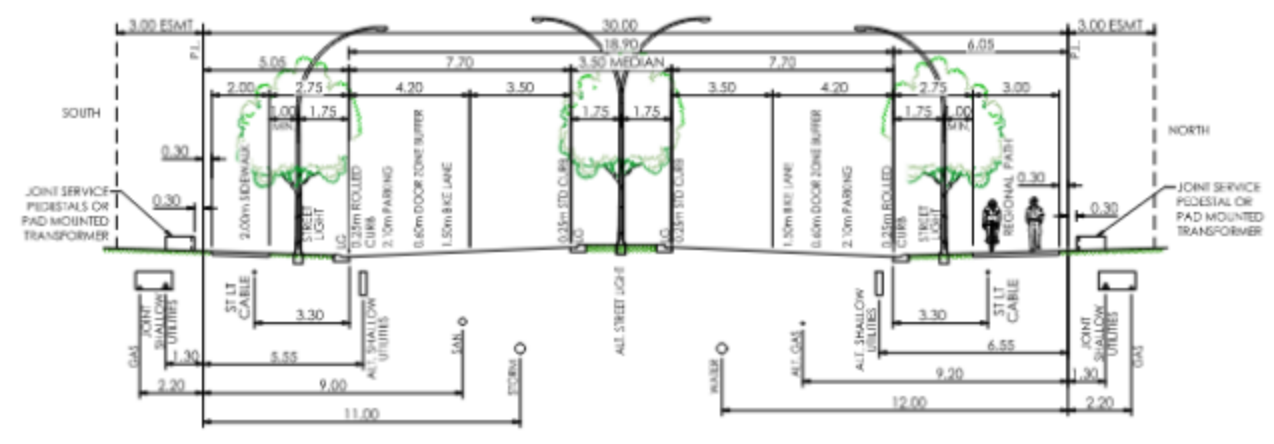
30.0m MODIFIED PRIMARY COLLECTOR 2.0m SEPARATE WALK ONE SIDE / 3.0m REGIONAL PATH ONE SIDE 1:200
